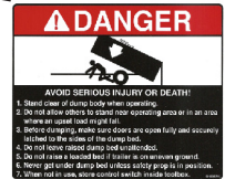
Part 080012B Locate in an easy to read location here and on opposite frame
